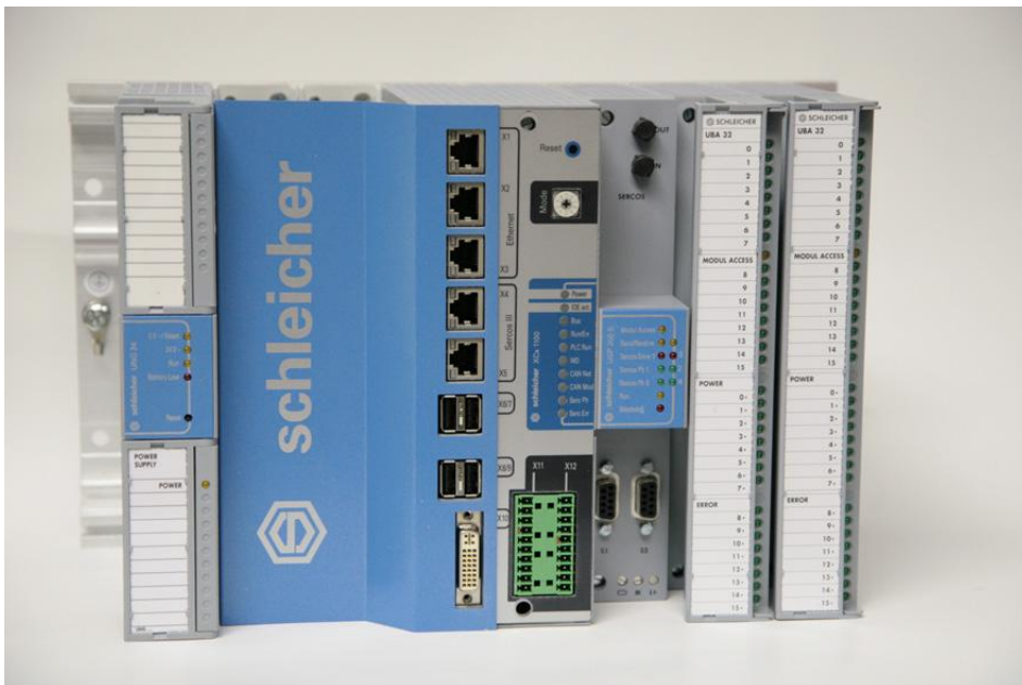
Illustration: Schleicher's XCx 1100 high-performance controller features a Sercos III interface
